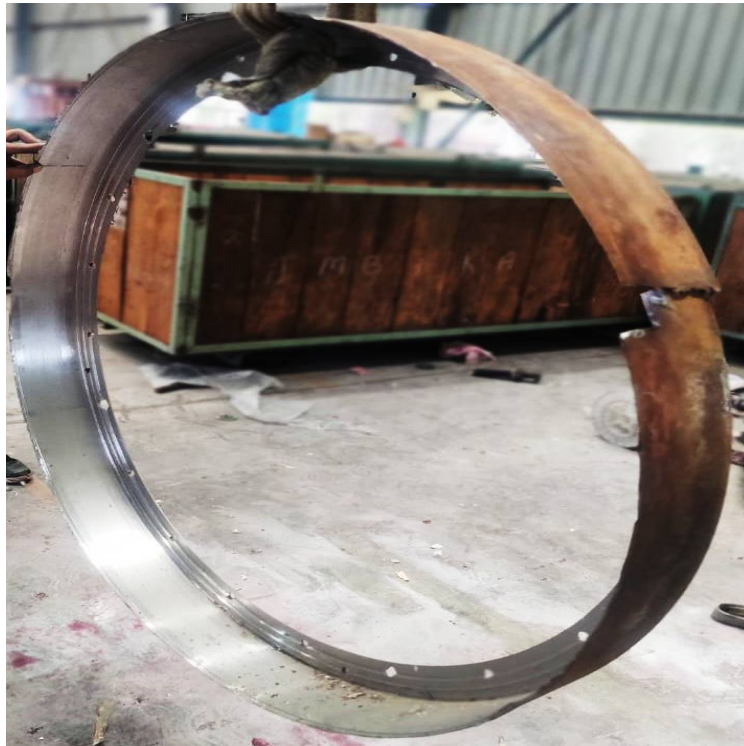
Fig.1. Labyrinth showing cracking on weld joints.
