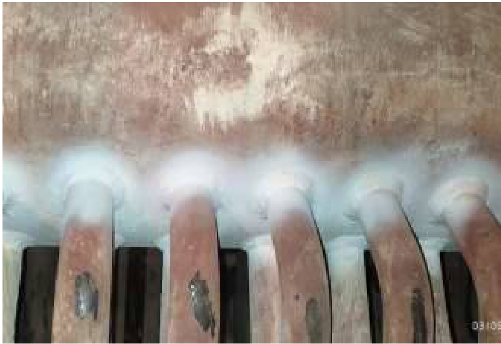
Figure 4 DP testing of FSH Stub joints
