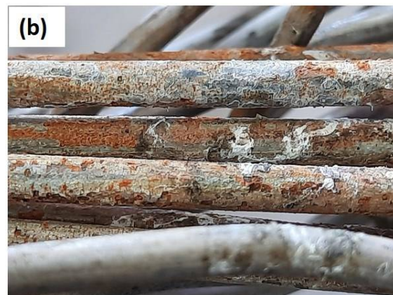
Fig-13. Photographs of ACSR conductor indicating corrosion of strands (a) Aluminum strands (b) steel strands
