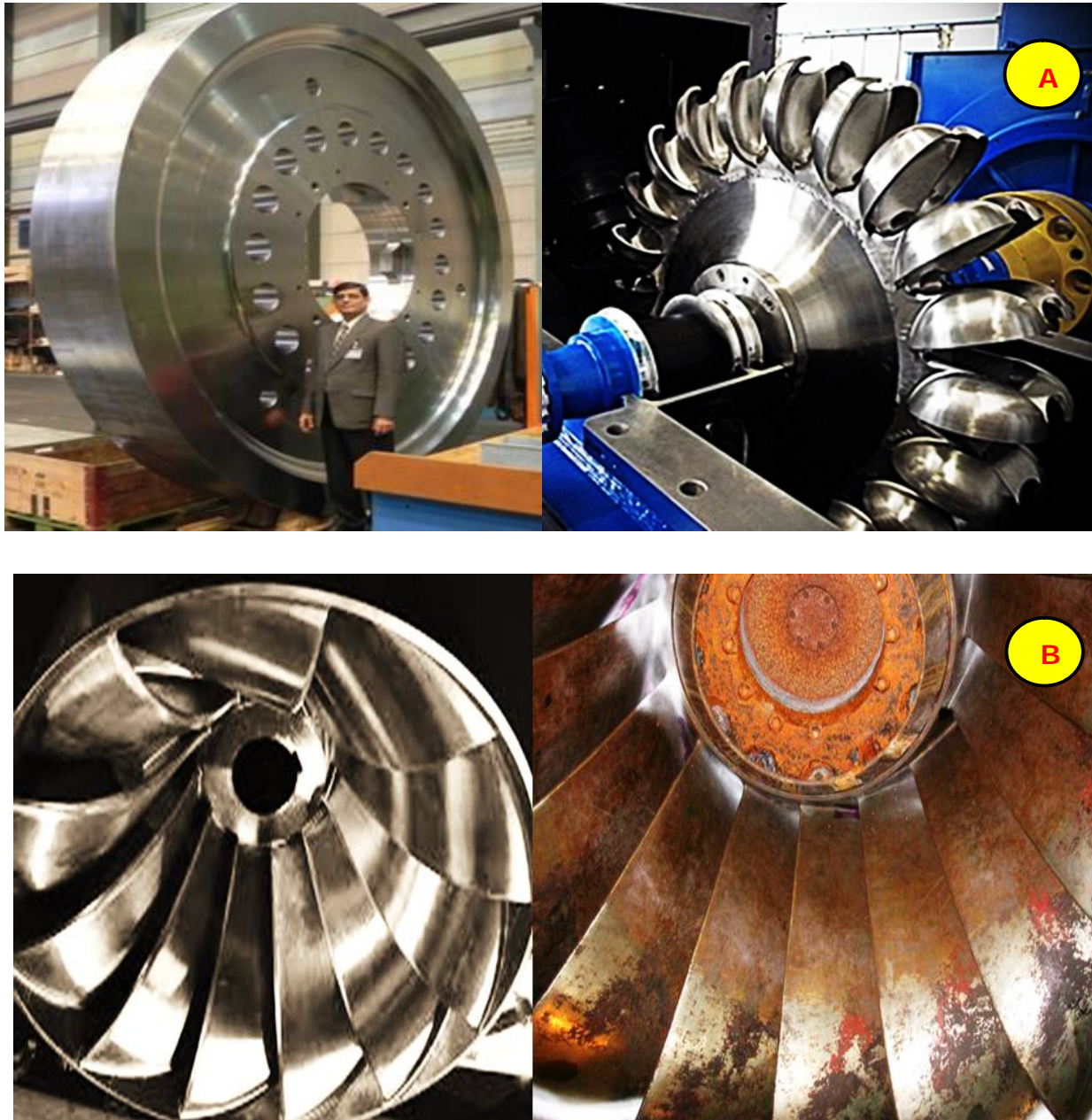
Fig.1. Hydro turbine appearance and role of metallurgy can be seen here a) Pelton Turbine and b) Francis Turbine.
