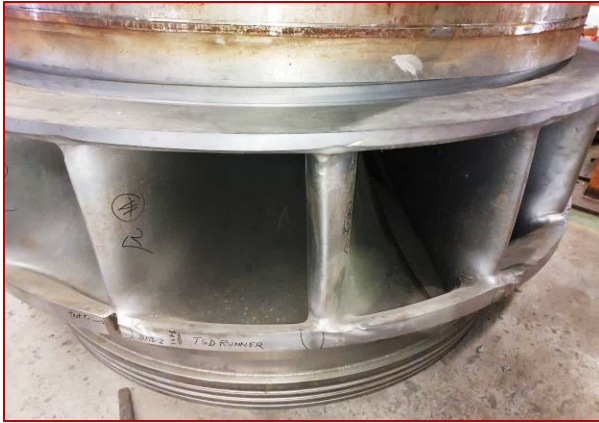
Fig.3: Francis Turbine Damage due to cracking and erosion.
