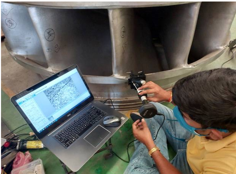
Fig.6: Francis Blades are under metallurgical examination.
