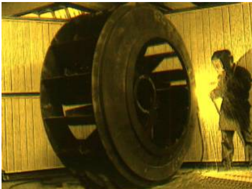
Wear protecting a rotating device, such as Fan Blades, include weight
